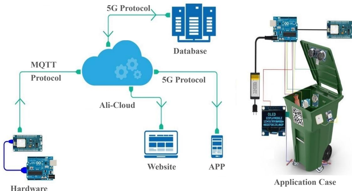
**Figure 5-2 Workflow of the Smart IoT module**
