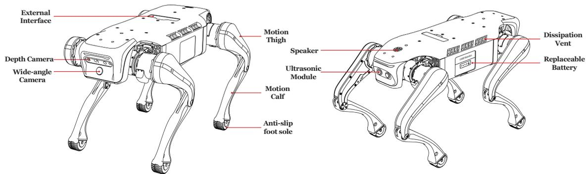
**Figure 4-3 Hardware peripherals of the quadruped robot**
