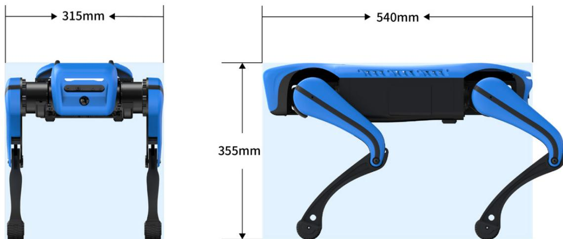
**Figure 4-1 Configuration dimensions of the quadruped robot**
